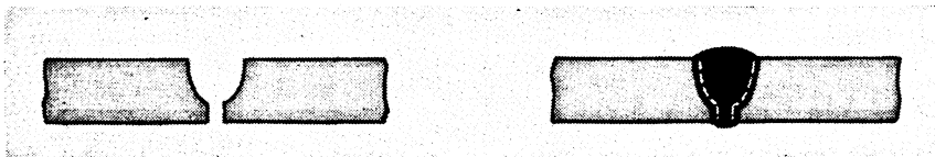
FIGURE 73.—Open single-U butt joint.
