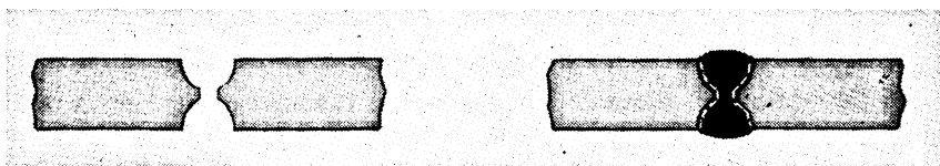
FIGURE 74.—Open double-U butt joint.
