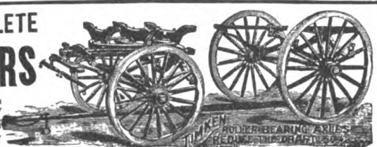
Trussed Platform Wagon Gear Complete, Ready for Body.
