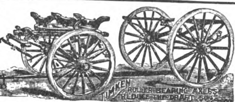
Trussed Platform Wagon Gear Complete, Ready for Body.
