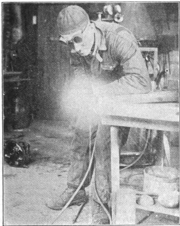
Figure 1. Forming the V-groove with the Cutting Torch.
