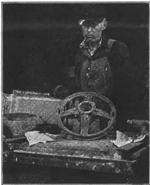
Fig. 3. The Welded Casting Showing the Location and Extent of the Weld
