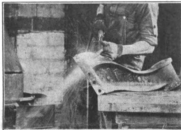
Fig. 2. The Welding Position of the Casting; the Torch in Operation.
