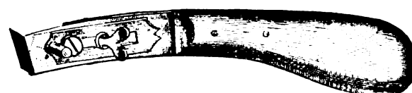
Special Knife Used for Cutting Groove for Charlier Tips.
