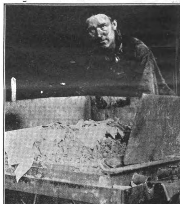
Fig. 2. Covered with Asbestos for Slow Cooling.
