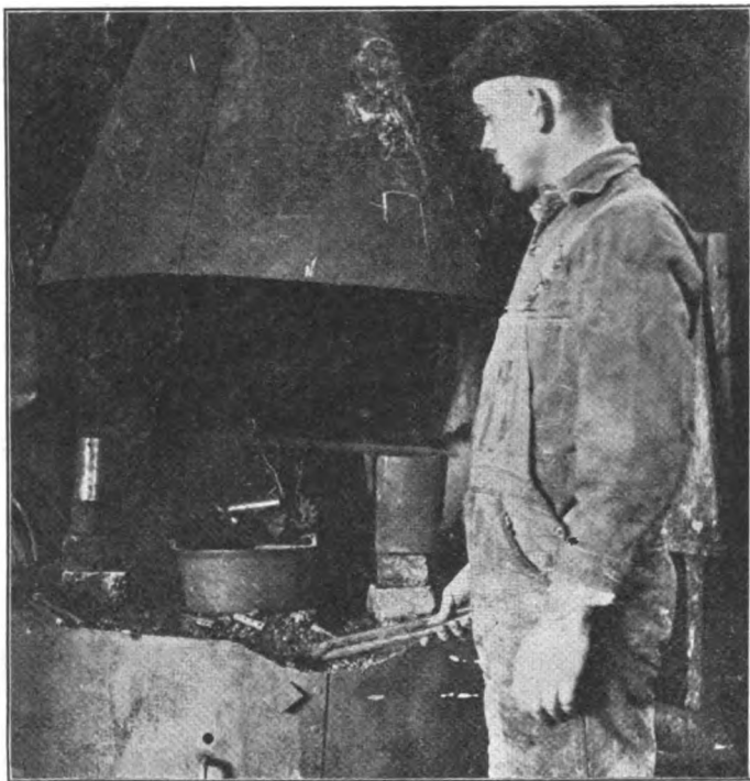
Fig. 3. Cyaniding Several Articles at One Time.
