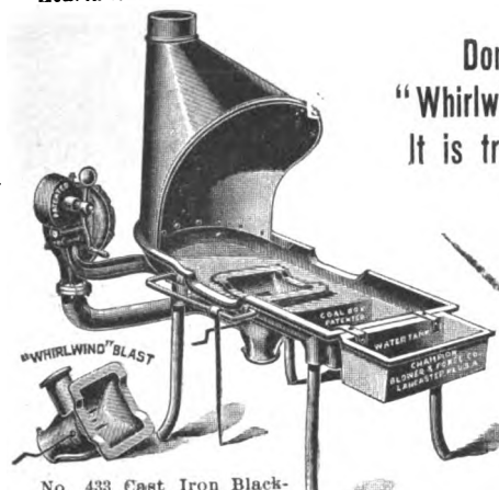
No. 433 Cast Iron Blacksmith's Forge with Half Hood and Sloop Bottom Coal Box. Hearth 32x46 in. Fan 12 in. in diameter.
