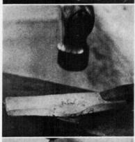
Take a NEAR WELDING heat and split this lip down the middle with a hot chisel to form a semi-circular pocket to receive the fan-shaped scarf on the piece which will be welded in.
