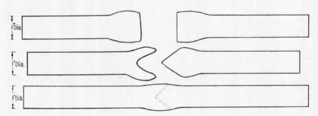
Take a NEAR WELDING heat on the end of one bar and upset to about 11 times the original size. This can be done by tamping as shown here—
