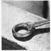
While it is still hot, dress up the eye on the bick and then the shank on the anvil face with the shoulder of the eye over the rounded edge.
