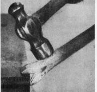
Take a NEAR WELDING heat on the second bar and upset the end a little less than the first bar.
