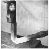
Continue working up the bend like this, keeping a full inside radius and finishing the outside corner to a sharp square edge.
