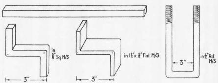
To make the **Z** or cranked bends, mark the  $\frac{4}{3}$ " square and  $1\frac{1}{2}$ "  $\times \frac{2}{3}$ " flat as described on page 78, paragraph (b) allowing half the thickness of the metal for each bend.
