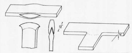
Take a NEAR WELDING heat on the middle of the piece which forms the top of the T. Upset to 1½ times the thickness with extra metal on one edge of the bar to form a bulge like this—
