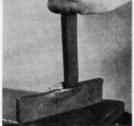
Take a NEAR WELDING heat on the end of the piece which will form the leg of the T and upset it for about  $\frac{1}{2}$ ".
