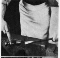
Flatten the end a little and make a double wing-shaped scarf by working over the rounded edge of the anvil.
