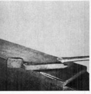
To retain the maximum strength in the boss the rivet holes should be punched, not drilled. Start to punch as shown with the shoulder downwards over the edge of the anvil.
