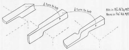
To forge a pair of tongs, cut off a piece 12" long from a  $\frac{7}{8}$ " square bar.
