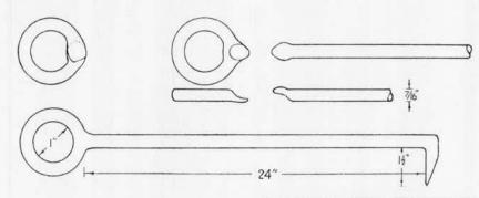
To make the shank cut off 26" from a 76" round with a cold chisel.
