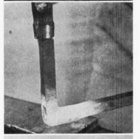
The completed bend should have a square outside corner and a good inside radius as shown here.
