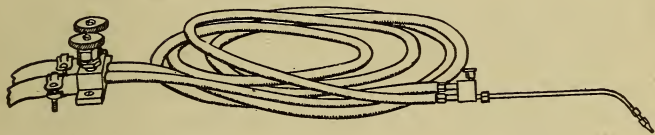
Figure 273.—Type of Light Blowpipe Suitable for Welding Sheet Aluminum, Lead Burning, Etc., Showing Bench Block at the Left.
