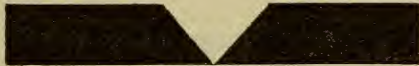
Figure 251.—Bevel Employed on Metal Less than \frac{5}{8} or \frac{3}{4} Inch and Over \frac{1}{8} Inch in Thickness.
