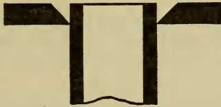
Figure 271.—Preparation of Flange to Be Welded to Thinner Section Plate.
