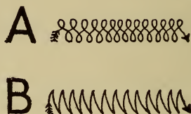
Figure 259.—Two Correct Movements to Give the Welding Flame. A , Figure 8 Movement, Best Suited to Ordinary Work; B , Zigzag Movement, Which Some Operators Prefer.
