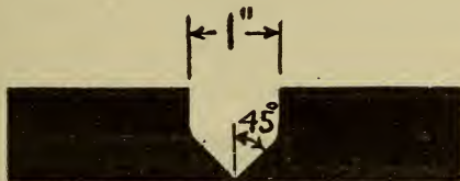
Figure 253.—Beveling of Sections Over \frac{3}{4} Inch in Thickness Where Parts Must Be Welded from One Side Only.
