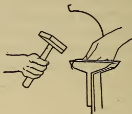
Figure 185.—Bending Hook on Wire Ball, Showing Use of Creasing Stake.
