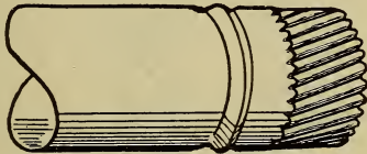
Figure 62.—Showing Crimp and Bead Made with Crimping and Beading Machine.
