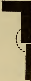
Figure 269.—Dotted Line Shows How Filling Material Must Be Built Up When Welding Angle to Thinner Section Plate.
