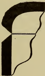
Figure 263.—Location of Joint When Welding Convex End to Steel Cylinder.
