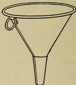
Figure 195.—Common Funnel, in Which Both Body and Spout Are Frustums of Cones.
