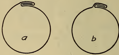
Figure 153.—Pipe Seam Hooked Together and Grooved.
