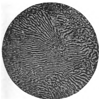
FIG. 64.—Pearlite (Stead) \times 1,000 .
