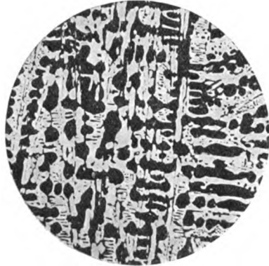
FIG. 70.—White Cast Iron (Longmuir). Cementite (white), Pearlite (dark). × 150.
