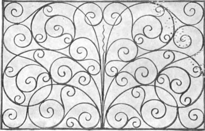
*Fig. 70. Grille of Flat Scrollwork*
