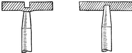
*Fig. 17. Completing the Punch Hole*
