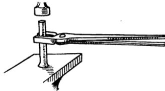
*Fig. 13. One Method of Upsetting*
