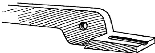
*Fig. 6. Jaw with Fuller Mark*
