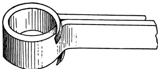
*Fig. 43. Fitting the Prongs in an Eye Weld*
