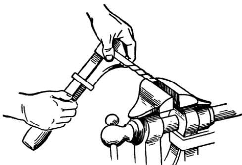
*Fig. 44. Twisting a Bar*
