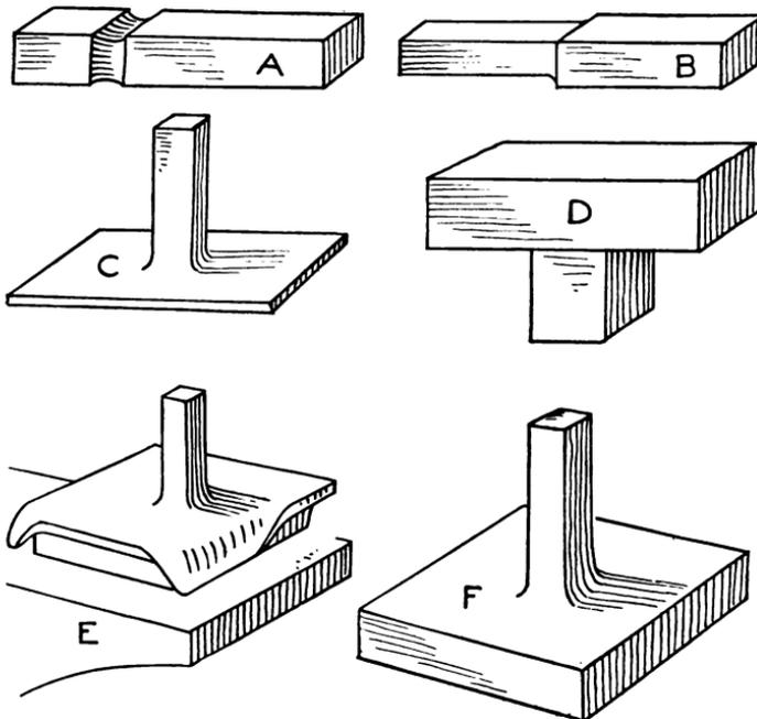
*Fig. 79. Method of Forging a Base*
