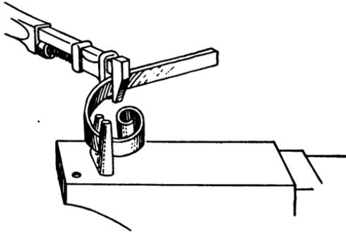
*Fig. 68. Forming the Body of a Scroll*
