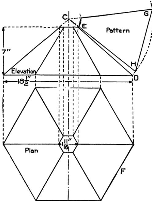
*Fig. 117. Drawing for Shade of Electric Lamp*
