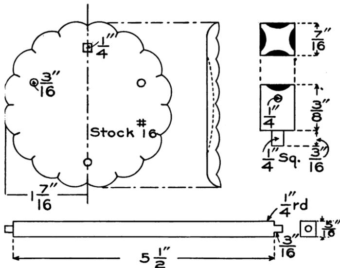
Fig. 109. Drawing for a Pull with Scalloped Plate
