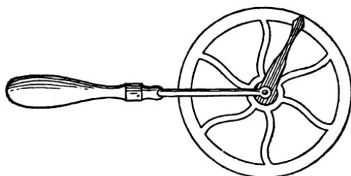
Fig. 21. *Traveler, or Tire-Measuring Wheel*
