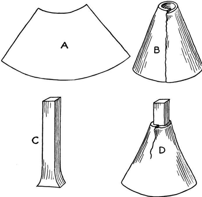
*Fig. 81. Method of Making Base for Candlestick*
