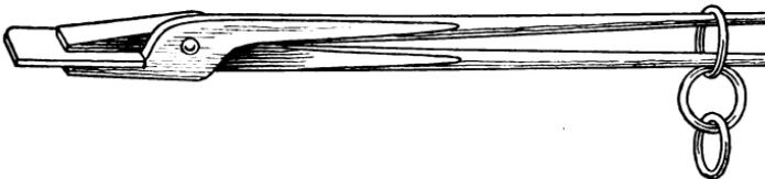
*Fig. 8. Binding the Tongs with a Ring*
