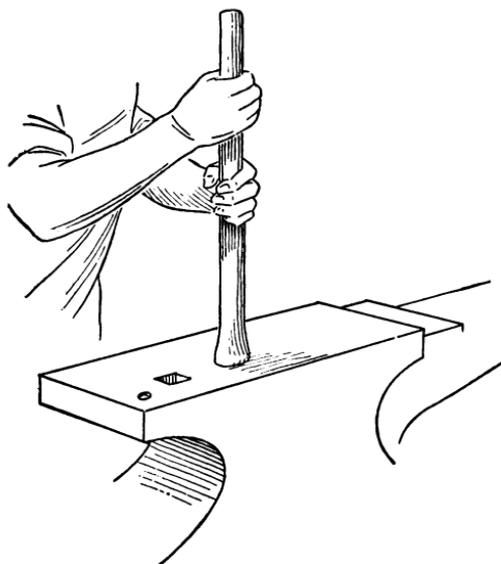
*Fig. 15. Upsetting by Ramming*
