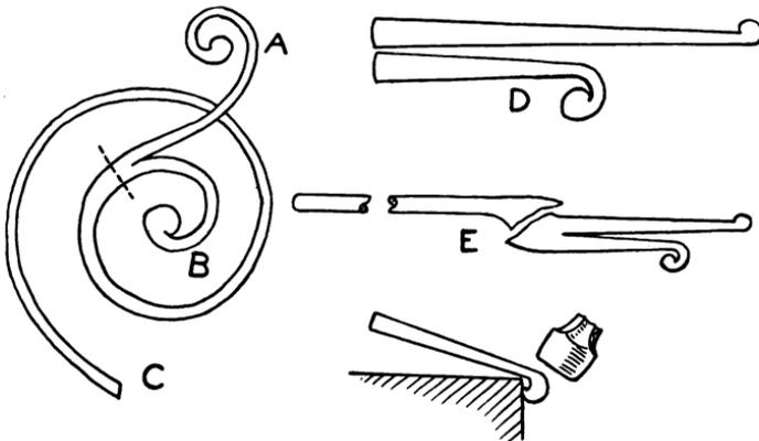
*Fig. 76. Method of Welding Scrollwork*
