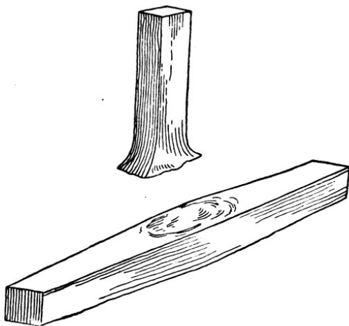
*Fig. 37. Stock Prepared for a T Jump Weld*
