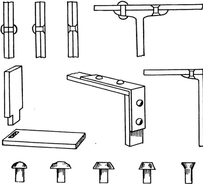
*Fig. 63. Methods of Riveting*
