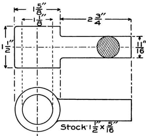
Fig. 41. Welded Eye from Flat Stock
