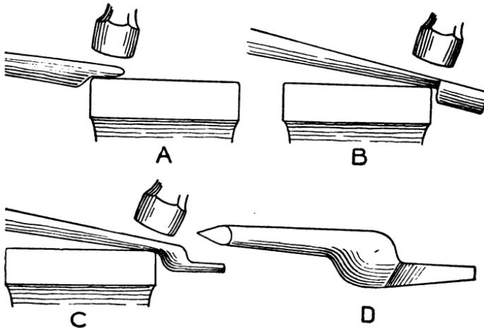
*Fig. 5. Method of Forging Tongs*
