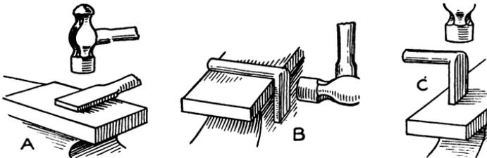
*Fig. 107. Making the Handle of a Drawer-Pull*
