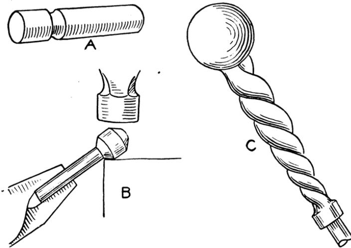
*Fig. 59. Working Up a Ball*
