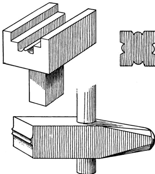
*Fig. 46. Section of a Twisted Bar and Tools Used in Swaging*
