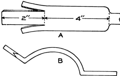
*Fig. 42. First Steps in Making an Eye Weld*
