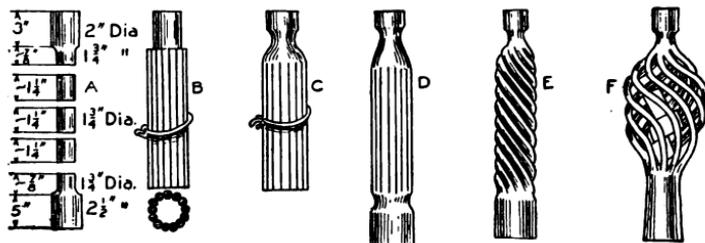
Fig. 55. Method of Forging the Bulb
