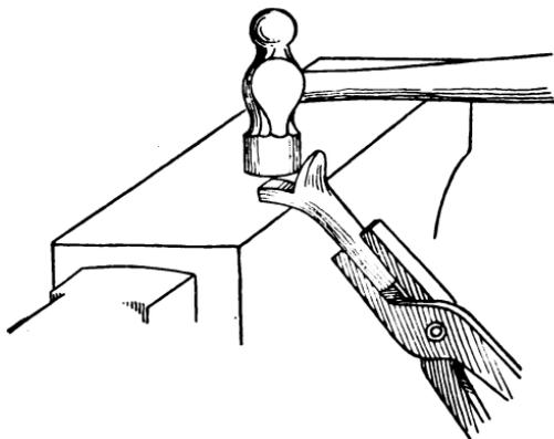
*Fig. 27. Forming Scarfs to Fit Bar*
