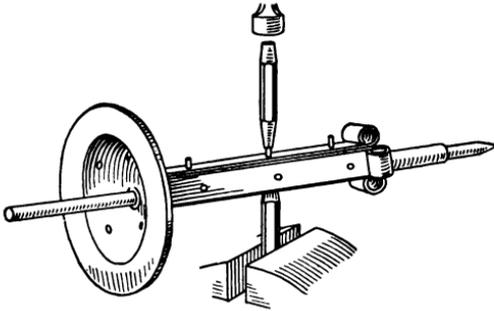
*Fig. 120. Riveting the Braces*
