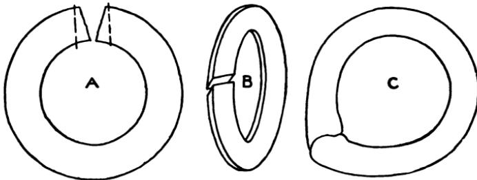
Fig. 39. *Welding Flat Rings*
