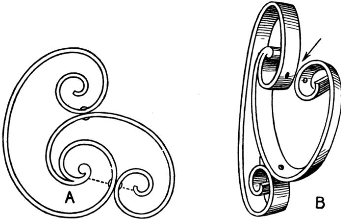
*Fig. 75. Method of Riveting Scrollwork*
