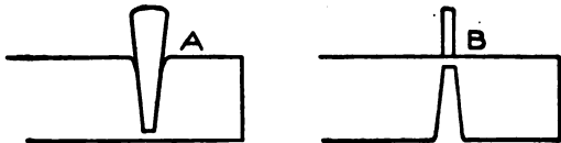
Fig. 160. Method of Cutting Off Hot Stock
