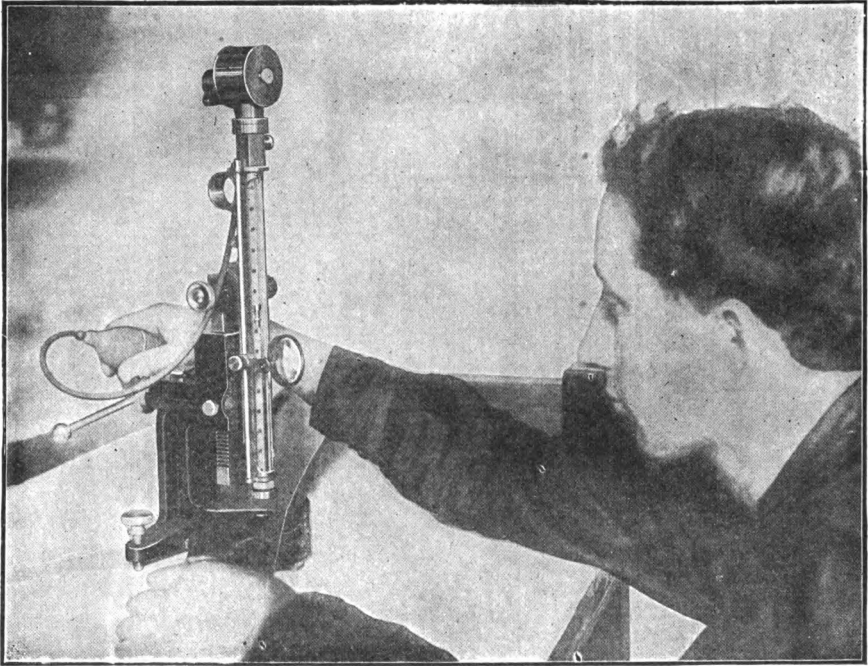
Fig. 188. Method of Testing Sheets and Flats Courtesy of Shore Instrument Company, New York City
