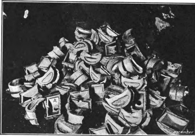
Fig. 13. A Heap of Finished Forged Coupler Pocket Filling Blocks
