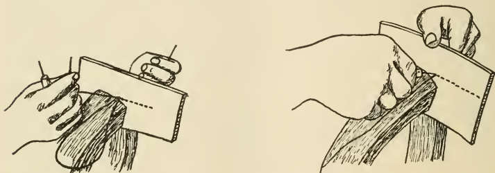
FIG. 234.—STITCHING WORK HELD IN SEWING HORSE.
